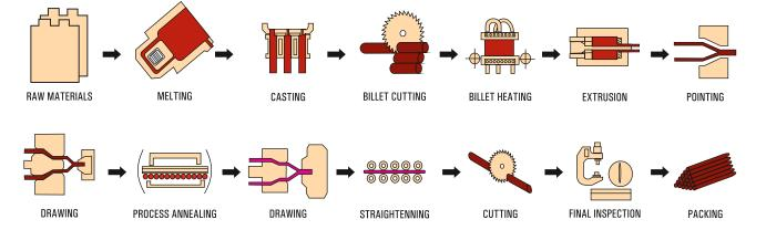
Nippon ACR Copper Tubes & Coils are Bright Annealed having uniform grain size, controlled hardness, elongation & tensile strength. Tube can easily bend & brazed. Our tubes are good heat exchanger, leakproof, reliable & long lasting for following specifications
